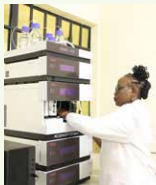
Patropa Jepkurui with a High Performance Liquid Chromatography machine at the science lab
