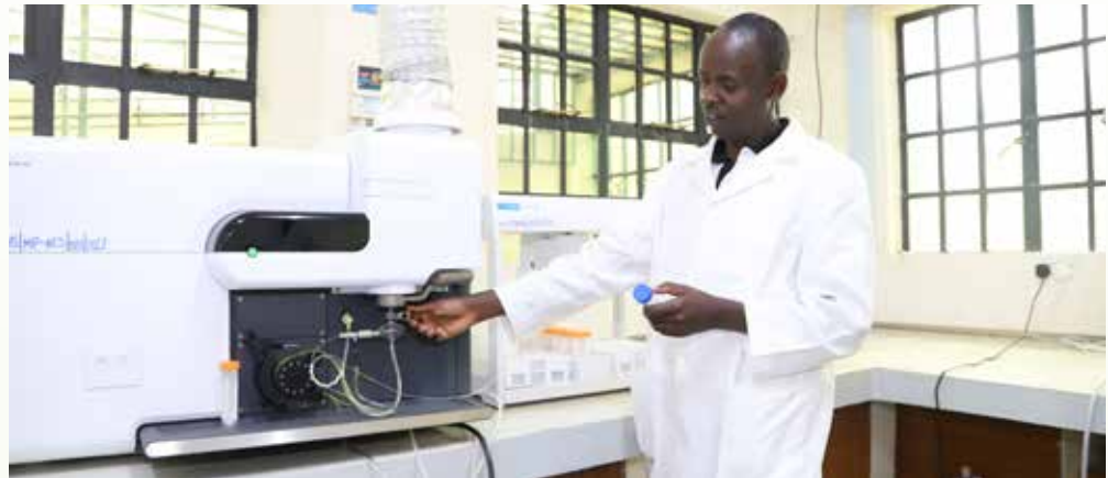
Charles Gitau with a Microwave Plasma Atomic Emission Spectroscopy (MP-AES) machine at the science lab
