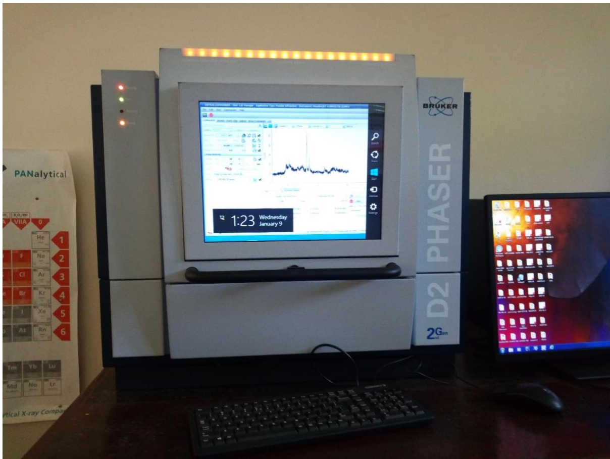
XRD Instrument Bruker D2 Phaser model at the department of Geology and Mines, Ministry of Petroleum and Mining.
