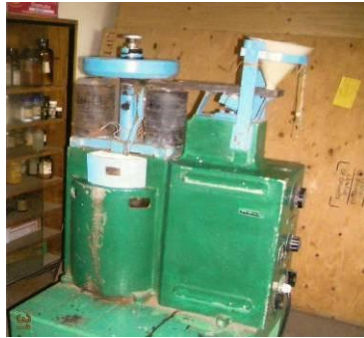
Plate 3. 2 Laboratory Magnetic Separator at the lapidary Laboratory Mines and Geology Department of Ministry of Environment and Mineral Resources.
